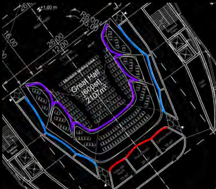
Sound diffusion and sound absorption distribution
